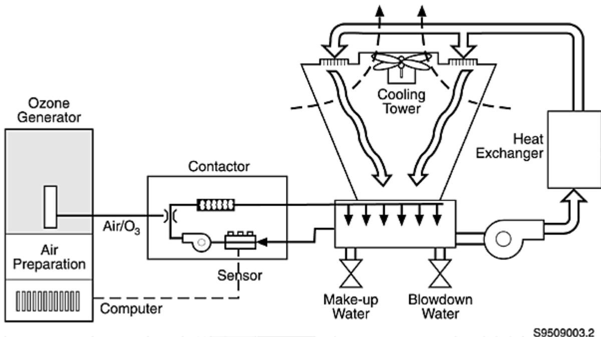
**Fig. 2. Process for Ozone Treatment of Cooling Tower Water**
