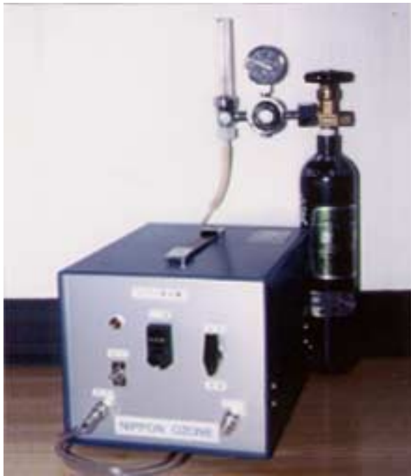
Fig. 1. Ozone generating system.
