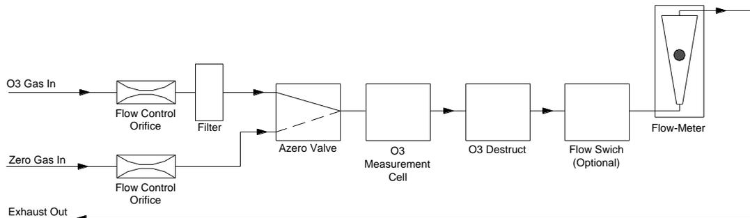
Figure 10-1: Pneumatic Diagram
