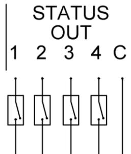
**Figure 4-8: Status Output Schematic**
