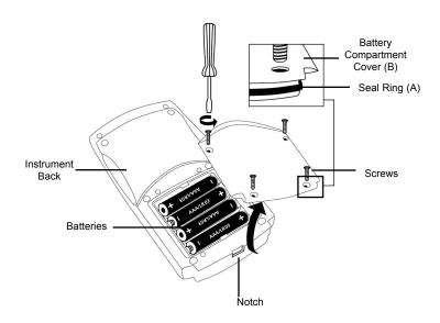
To ensure that the instrument is waterproof:
