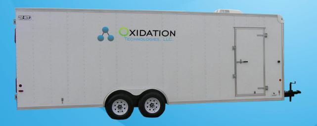
Ozone Trailer Systems are used for groundwater remediation applications. The trailer houses all equipment for a safe and portable system that are completely automated. Trailer systems can be provided using our custom steel trailers that are a step above the standard cargo trailer you have seen in the past.
