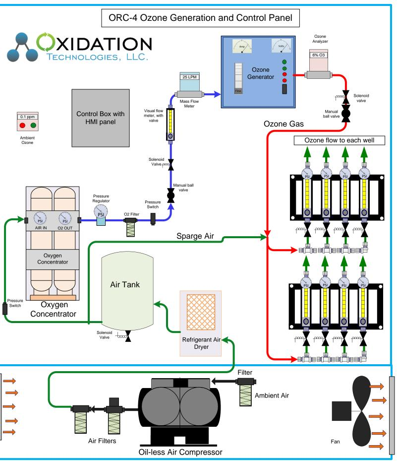
System installed in one enclosure.
