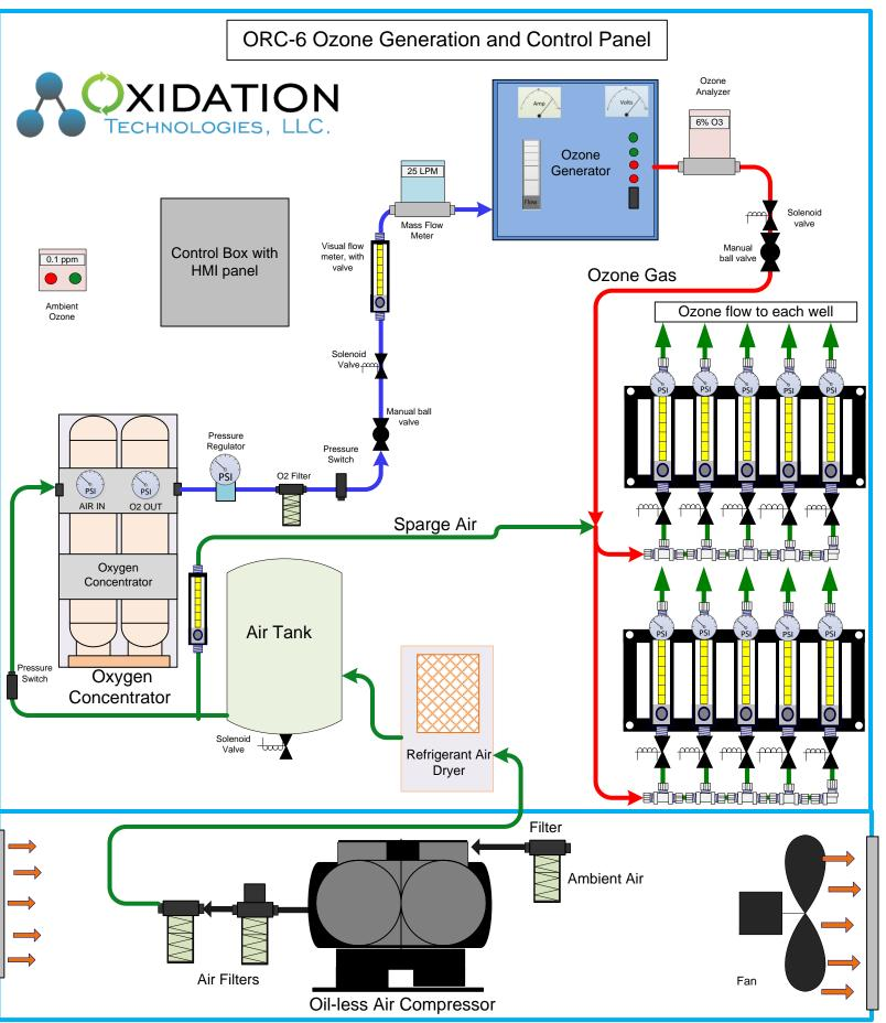
System installed in one enclosure.
