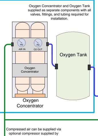
Oxidation Tech, or customers existing compressed air source.
