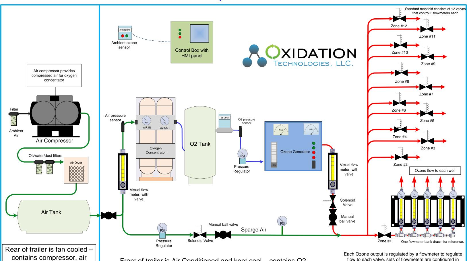
Front of trailer is Air Conditioned and kept cool – contains O2 concentrator, O2 tank, O3 generators, manifold and control system.
