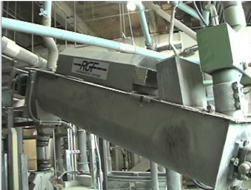
Tempering auger with UV/Ozone photo-ionization hood mounted
