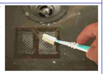
3. **NOTE:** Try to be very careful not to remove the screen from the mica. If the screen comes off the mica sheet this can be repaired by first cleaning the mica with alcohol and then putting a very thin amount of silicone on the existing silicone that is stuck to the screen then re place them on the mica in the same position as it was originally.
