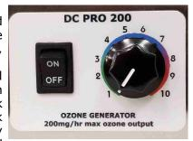
indication that the generator is set right is when you come home after being away for 6-8 hours and smell just a hint of the sweet fresh smell of ozone. If strong ozone is smelled, simply turn the output level control down. This is a case where more is not considered better. The levels of ozone required to deodorize most environments are from .03 ppm to .1 ppm.
