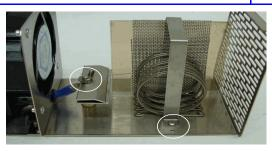
4. Once the plate hold down bracket and HV contact bar are removed, remove the plates by lifting them straight up as shown.
