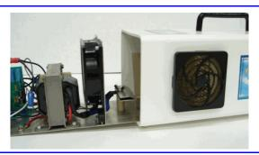
3. Remove the two Philips screws from the plate hold down bracket and the wing nut from the HV clamp as indicated.
