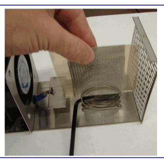
8. Re install the HV clamp and plate hold down bracket that was removed in step 2.
