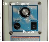
is more ozone present than is required to do the job. A good indication that the generator is set right is when you come home after being away for 6-8 hours and smell just a hint of the fresh sweet smell of ozone. Simply turn the output level control down. This is a case where more is not considered better. The levels of ozone required to deodorize most environments are from .03 ppm to .1 ppm.
