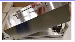
3. Remove the top support bar by removing to 2 Philips (star) screws circled in the image.
