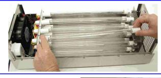
6. To remove the second and third row of tubes you will need to first remove the tube support bracket after removing the tubes. This bracket is removed by removing 2 screws from each as indicated in the image. Then repeat the removal of the hold down brackets, ties, and tubes as in step 4, 5, & 6 for 2<sup>nd</sup> and 3<sup>rd</sup> rows.
