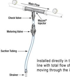
Installed directly in the main flow line with total flow of the system moving through the injector.
