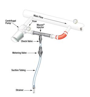
Installed in conjunction with a centrifugal pump to boost pressure through the injector thereby creating a differential pressure and producing a vacuum for chemical induction downstream from the pump.
