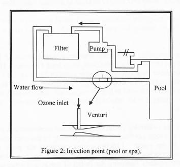
Figure 2 shows a suitable ozone injection point for pools or spas using a venturi. It is normally fitted before the water outlet(s). A venturi inlet is often used to aerate spa water and may be obtained from pool and spa suppliers in a range of sizes to accommodate different flow rates and pipe diameters. When correctly installed, the flow of water through the venturi creates a
