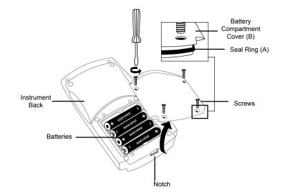
To ensure that the instrument is waterproof:
