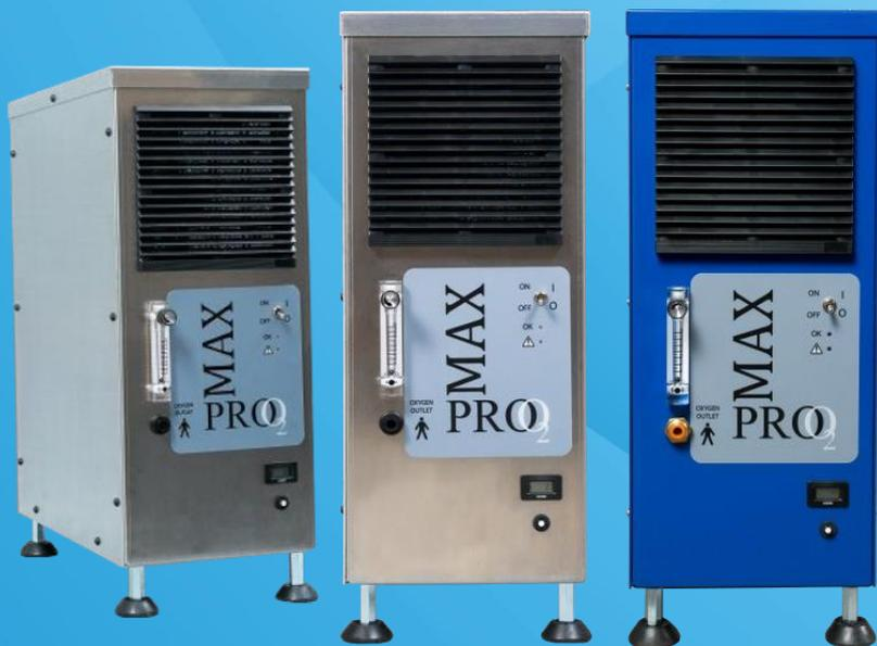
The MAX Series Oxygen Generators are perfect for industrial and commercial applications and delivers 90% purified O<sub>2</sub>. Built in a lightweight enclosure and designed with a built-in moisture separator to remove any water vapor before it enters the sieve beds. This allows for increased O<sub>2</sub> purity, and also maximizes the life of the sieve beds.
