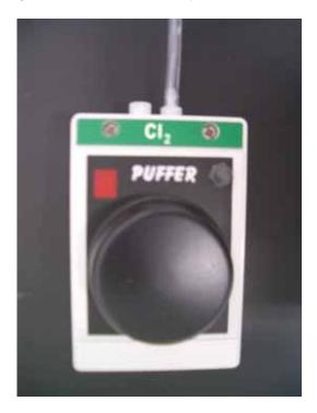
**Puffers** are water resistant for use in any environment and are designed to intrinsic safety standards. Generator cells provide hundreds of tests, with an LED to indicate the remaining life of the generator cell. Generator cells are easily changed, and the life indicator can be reset when a new generator is installed.
