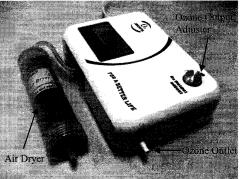
The power switch to turn on the power of the unit is at the left side of the generator. The air inlet is at the front side of the generator. The ozone output adjuster is to adjust ozone output. The control panel is on the top side of the unit.
