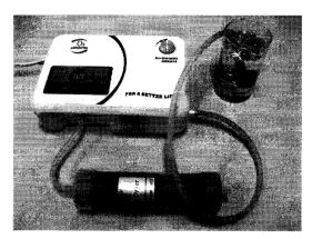
For any liquid treatment, place the unit at least 10cm above the liquid's surface to prevent it from entering the generator. For air treatment it is recommended to run without the hose connecting to the ozone outlet.
