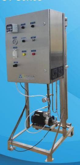
This Ozone Injection System is the Stainless Steel version of our OXS Ozone Water Systems and is made completely out of Stainless Steel components. Ozone is produced from an integrated oxygen concentrator and will produce 10 to 100 g/hr in water flows up to 100 GPM. The OST system is designed for point of use (POU) applications where high levels of ozone in water are required.
