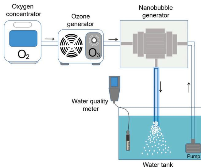
**Fig. 1.** Laboratory set up of NB-O<sub>3</sub> system in this study. Oxygen from the oxygen concentrator was fed into an ozone generator with a flow rate of 1 L/min. The generated ozone was then diffused with water inside the nanobubble generator and returned to the tank. Water parameters were measured using a multiprobe water quality meter.
