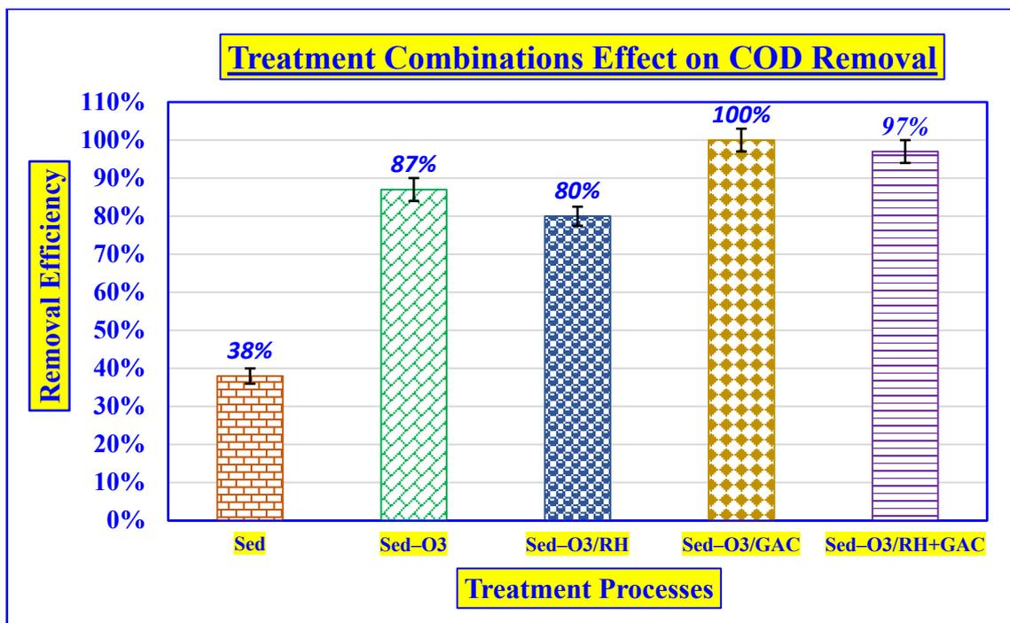
**Figure 4.** COD removal by different combinations (Initial COD= 490 mg/L; O<sub>3</sub> = 82.5 ± 2.2 mg/L; peristaltic pump speed = 150 rpm; C. T= 18 min; GAC= 400 g; RH= 400 g; GAC + RH = 200 g +200 g; pH = 6.9 ± 0.2; volume = 4 L; T = 25 ± 2 °C).
