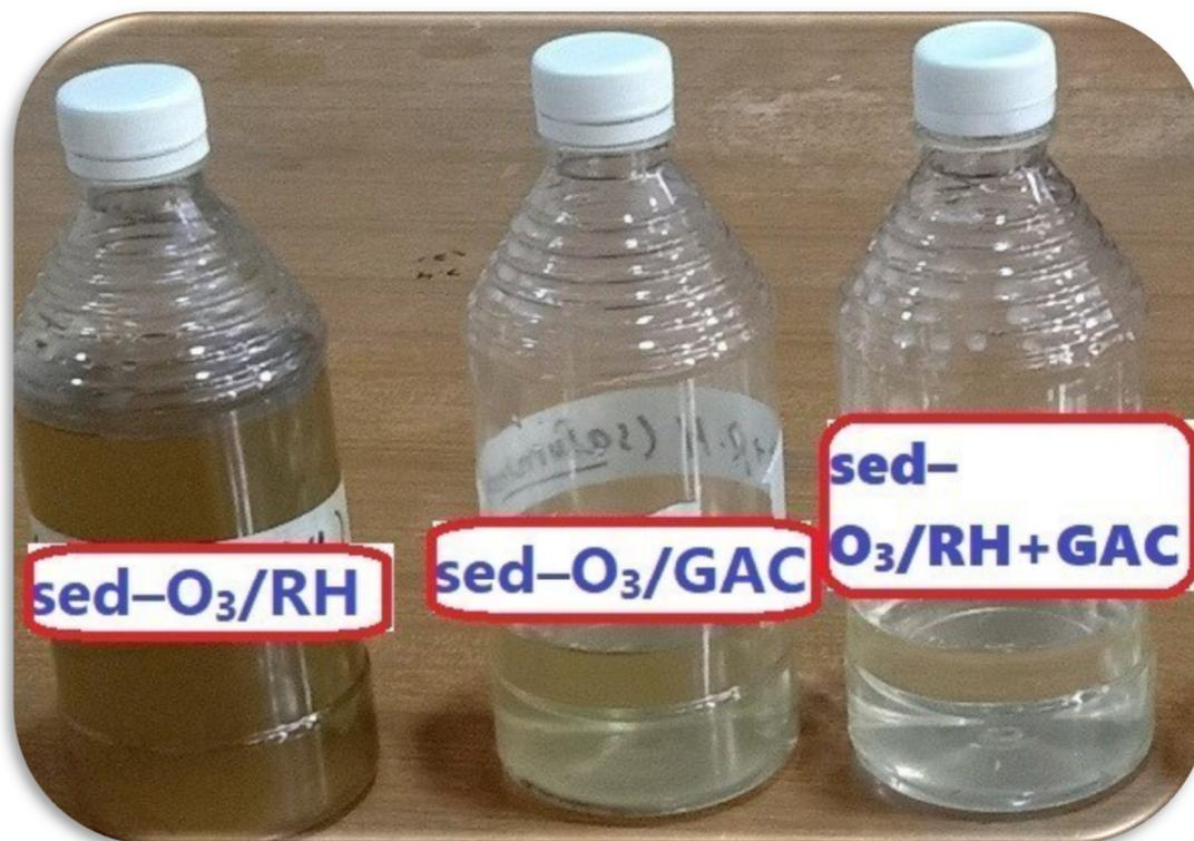
**Figure 5.** Treated samples of ASSWW by three treatment combinations.
