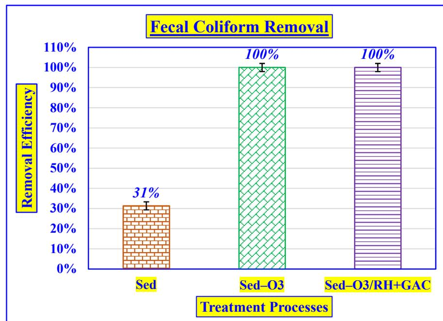
**Figure 10.** Fecal Coliform removal by hybrid system (Initial Fecal Coliform = 5170 MPN/100 mL; O<sub>3</sub> =  $82.5 \pm 2.2$  mg/L; peristaltic pump speed = 150 rpm; C.T = 18 min; GAC = 200 g; RH = 200 g; pH =  $6.9 \pm 0.2$ ; volume = 4 L; T =  $25 \pm 2$  °C).
