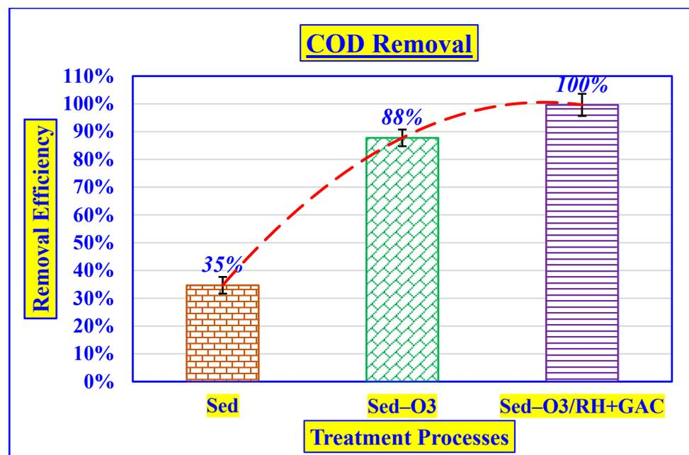
**Figure 7.** COD removal by hybrid system (Initial COD =  $490 \pm 11.5$  mg/L;  $O_3 = 82.5 \pm 2.2$  mg/L; peristaltic pump speed = 150 rpm; C.T = 18 min; GAC = 200 g; RH = 200 g; pH =  $6.9 \pm 0.2$ ; volume = 4 L; T =  $25 \pm 2$  °C).
