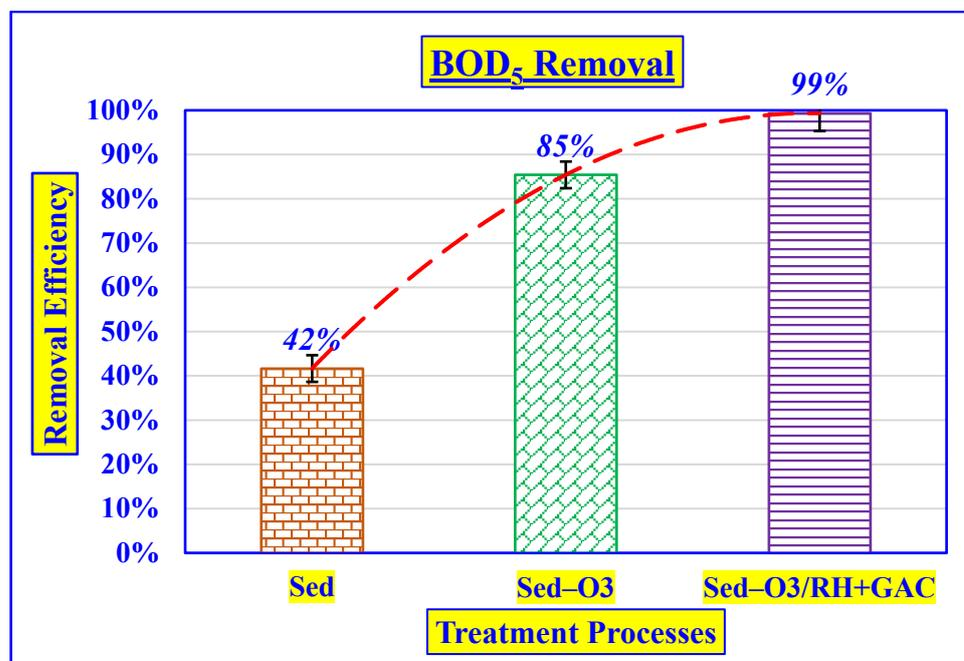
**Figure 8.** BOD<sub>5</sub> removal by hybrid system (Initial BOD<sub>5</sub> = 225 ± 9 mg/L; O<sub>3</sub> = 82.5 ± 2.2 mg/L; peristaltic pump speed = 150 rpm; C.T = 18 min; GAC = 200 g; RH = 200 g; pH = 6.9 ± 0.2; volume = 4 L; T = 25 ± 2 °C).
