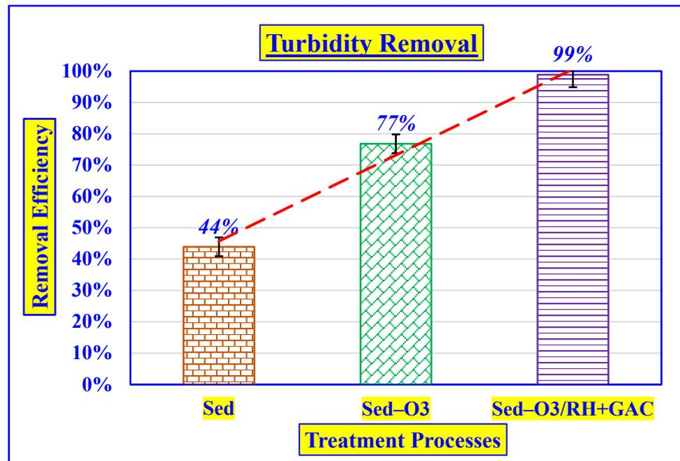
**Figure 6.** Turbidity removal by hybrid system (Initial turbidity =  $669 \pm 16$  NTU;  $O_3 = 82.5 \pm 2.2$  mg/L; peristaltic pump speed = 150 rpm; C.T = 18 min; GAC = 200 g; RH = 200 g; pH =  $6.9 \pm 0.2$ ; volume = 4 L; T =  $25 \pm 2$  °C).
