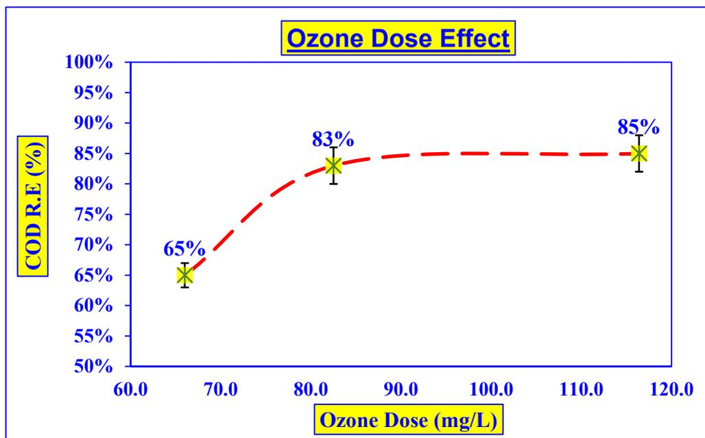
**Figure 2.** Ozone dose optimization in ozonation process ( $O_3 = 66.0 \pm 1.5$  mg/L,  $82.5 \pm 2.2$  mg/L,  $116.40 \pm 3.6$  mg/L; pH =  $6.9 \pm 0.2$ ; C.T = 15 min; volume = 4 L; T =  $25 \pm 2$  °C).
