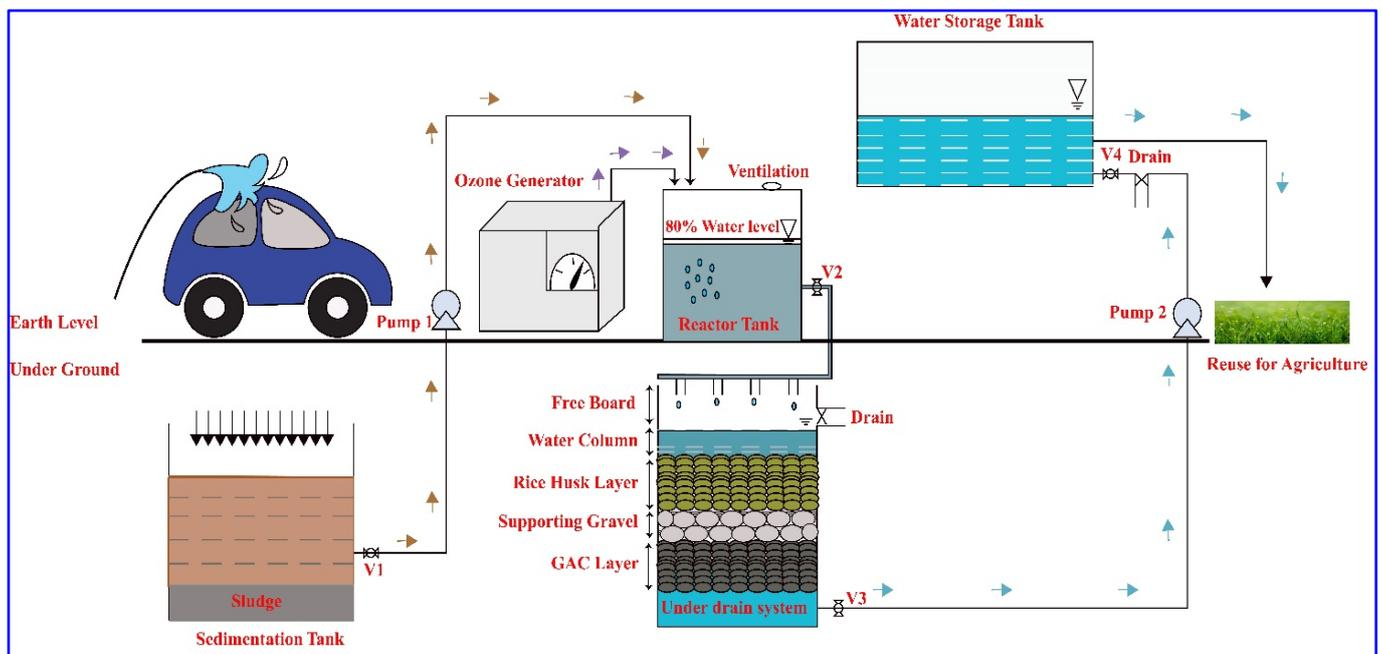
**Figure 1.** Schematic diagram of novel hybrid system.
