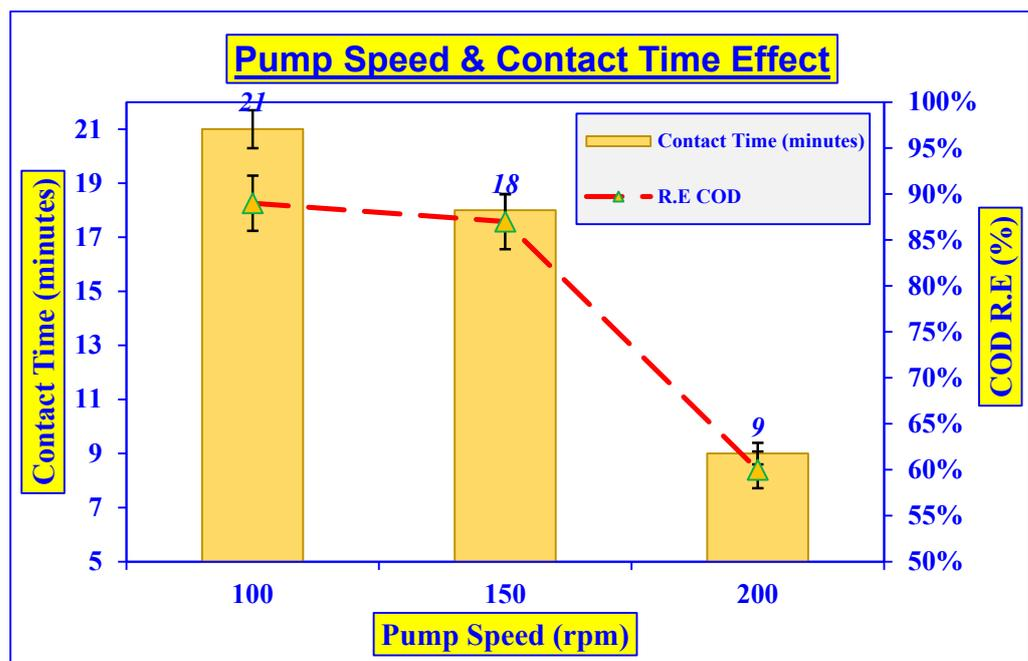
**Figure 3.** Pump speed and Contact time optimization in ozonation process (peristaltic pump speed = 100 rpm, 150 rpm and 200 rpm; t = 9 min, 18 min and 21 min; Initial COD = 490 mg/L;  $O_3 = 82.5 \pm 2.5$  mg/L; pH =  $6.9 \pm 0.2$ ; volume = 4 L; T =  $25 \pm 2$  °C).
