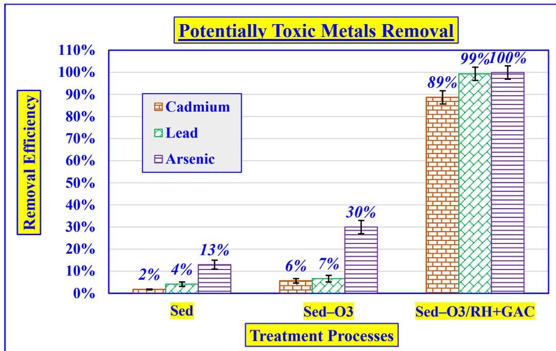
**Figure 12.** Toxic metals removal by hybrid system (Initial Cd = 0.056 mg/L, Pb = 0.012 mg/L and As = 0.1 mg/L; O<sub>3</sub> = 82.5 ± 2.2 mg/L; peristaltic pump speed = 150 rpm; C.T = 18 min; GAC = 200 g; RH = 200 g; pH = 6.9 ± 0.2; volume = 4 L; T = 25 ± 2 °C).
