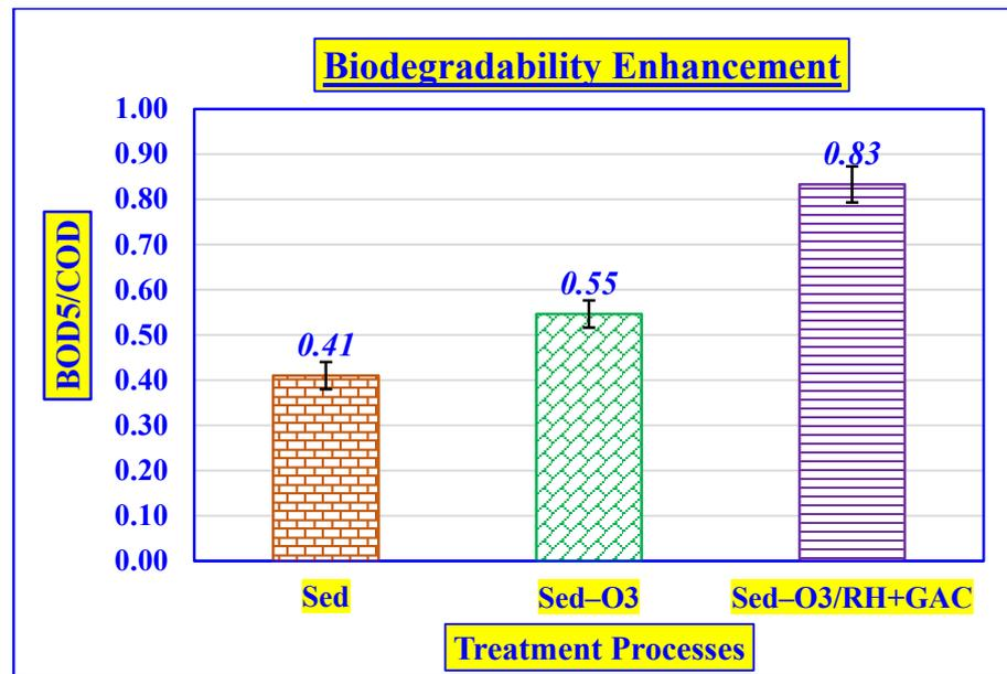
**Figure 9.** Biodegradability increased by hybrid system (Initial COD =  $490 \pm 11.5$  mg/L; Initial BOD5 =  $225 \pm 9$  mg/L; O<sub>3</sub> =  $82.5 \pm 2.2$  mg/L; peristaltic pump speed = 150 rpm; C.T = 18 min; GAC = 200 g; RH = 200 g; pH =  $6.9 \pm 0.2$ ; volume = 4 L; T =  $25 \pm 2$  °C).
