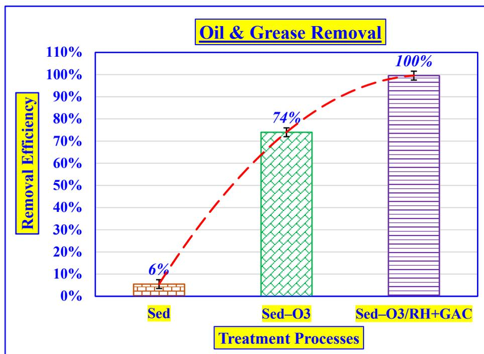
**Figure 11.** Oil and Grease removal by hybrid system (Initial O and G = 200 mg/L; O<sub>3</sub> = 82.5 ± 2.2 mg/L; peristaltic pump speed = 150 rpm; C.T = 18 min; GAC = 200 g; RH = 200 g; pH = 6.9 ± 0.2; volume = 4 L; T = 25 ± 2 °C).
