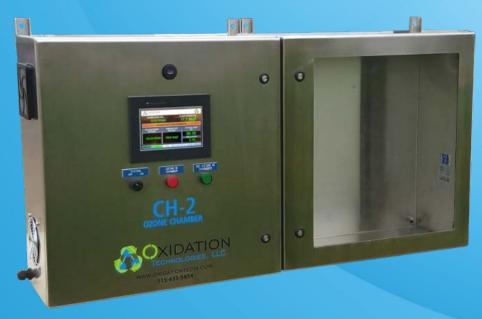
The CH-2 Ozone Chamber is a turnkey ozone environmental chamber with a range of 0-1,000 PPM. The chamber is automated and simple to use; perfect for testing objects to meet the required testing configurations.
