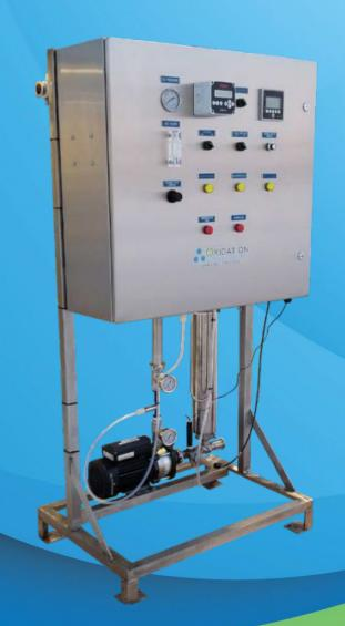
This Ozone Injection System is the Stainless Steel version of our OXS Ozone Water Systems and is made completely out of Stainless Steel components. Ozone is produced from an integrated oxygen concentrator and will produce 10 to 150 g/hr in water flows up to 100 GPM. The OST system is designed for point of use (POU) applications where high levels of ozone in water are required.
