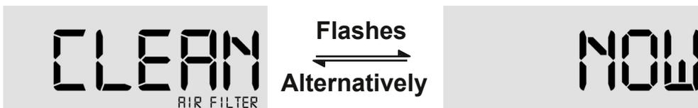
Pressing and holding the button for 10s will reset the countdown alarm total to 400H.
